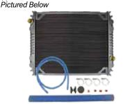
P/N 03-070200006 (Radiator Only) Copper Brass Radiator, 41.75"H x 30.625"W x 2.38" Thickness, 2.5" Inlet Upper Right @ 5.75", 2.5" Outlet Lower Right @ 5.75", 625" Dimpled Tubes On .4375" Centers, 15 FPI, Replaces OE 05-20514-001, A05-19870-003, A05-19870-021, BHTA9988, BHTC2315, BHTD9567, BHTE7236, BHTH5464, BHTU3698002, BTU3698001, DHTFR1306B0023, Fits 2003-2007, Pictured Below
