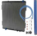
P/N 03-070263 (Radiator Only) P/N 03-070263K (Kit) Plastic Aluminum Radiator w/Frame, 42.125"H x 38.5" W x 2.1875" Thickness, 2.5" Inlet Upper Left, 2.5" Outlet Lower Right, Kit Contains (1) 36" x 2.5" Hose, (4) 2.5" Stainless Constant Torque Clamps, (1) Radiator Mount, (1) Set Bushings, (1) 6" x .378" Hose, Replaces OE 2400751, FRE47, FRRP80743B2, LT1191, Fits 2008-2011, Pictured Below
