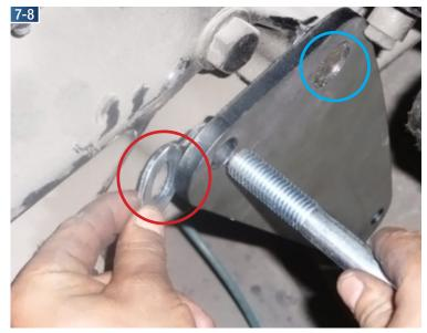
Install washer between frame and air cylinder mounting bracket.
